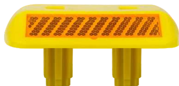
MODEL NO. : DA 52 Two Way Reflective Available with Single / Double / Without Shank Weight : 154 GM / 164 GM / 144 GM Dimensions : 100 x 110 x 20 mm Plastic body Reflective panel - Amber, Red or White
