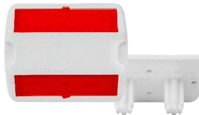
MODEL NO. : DA 54 Two Way Reflective Available with Single / Double / Without Shank Weight : 90 GM / 95 GM / 104 GM Dimensions : 100 x 80 x 20 mm
